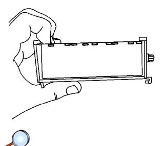
3. Spread the large tang side of the plastic bracket over the edge of the module. The bottom, undercut edge of the plastic bracket will snap over the bottom of the module when fully seated.
